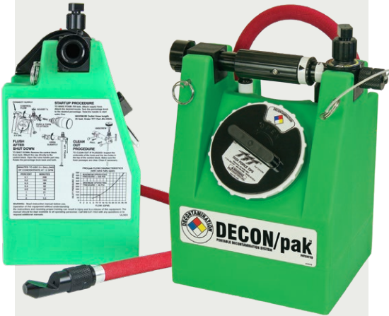
Flow is controlled by a twist grip valve that also functions as a carrying handle. Cleaning agents are added through the large, easy-open fill port that includes a debris screen.
