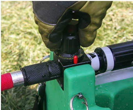
Large selector for agent proportioning from 0.1 to .5% for cleaning agent** or set to rinse with water only.
