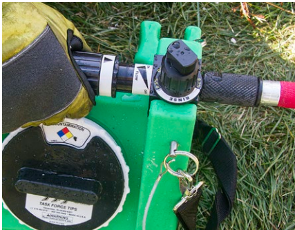
Flow is controlled by a twist grip valve that also functions as a carrying handle. Cleaning agents are added through the large, easy-open fill port that includes a debris screen.
