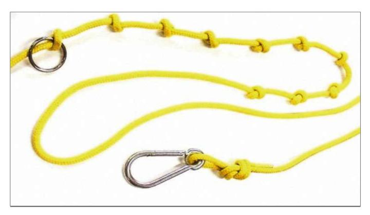
This is the end of the rope connected to the bottom of the bag (snap ring). This is a 200 ft. rope with 20 ft. ring/knot spacing. Finding 9 knots on a 200 ft. rope would indicate you have traveled 180 ft. of the 200 ft. of rope
