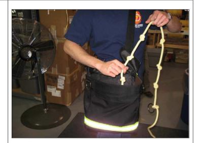
When the rope has been re-packed, close the top flap and place the snap hook put the side opening in the direction of deployment. Attach the snap hook on the ring or the shoulder strap.
