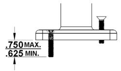
Tighten the screws to 15 in-lbs . DO NOT OVERTIGHTEN. Inserts may be re-used to reposition brackets or equipment
