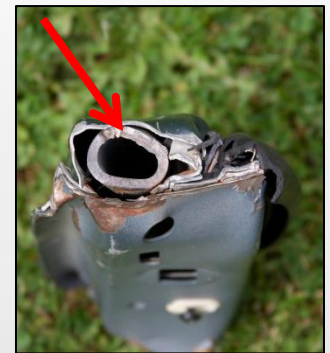
UHSS Reinforcing Tube. 280,000 lbs. of force to Make The Cut.
