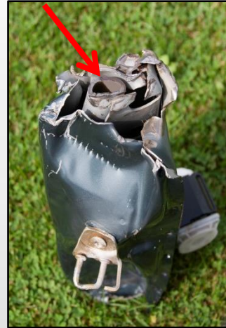
UHSS Reinforcing Tube. 280,000 lbs. of force to Make The Cut.
