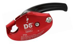
The D5 is a double-stop device with an auto-lock function, which is activated whenever the operator releases the handle; and a panic-brake function, which is not overly sensitive in normal use.
