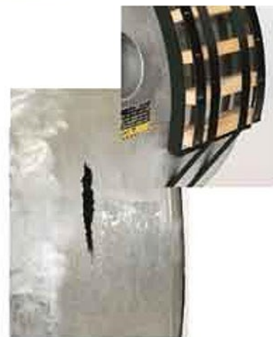
New Ladder Patch with 3/4" foam backing instead of 1/4" hard rubber
